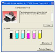
Figure 4-3. Maintenance Request Error Display on Status Monitor 3
