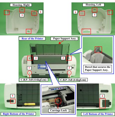
Figure 2-2. Paper Support Assy./Housing (left/right) removal
