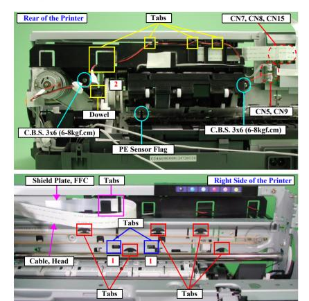
Figure 2-16. Holder, Shaft Assy. Removal (1)
