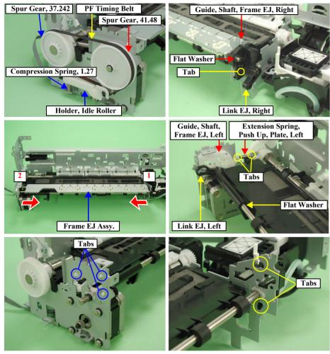
Figure 2-44. Paper Guide, Front/Roller EJ Assy. Removal (1)
