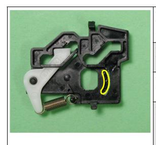
Contact point between the Guide Shaft, Frame EJ, Right and the Paper Guide, Front
