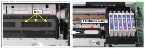
Figure 3-9. Setting the Thickness Gauge
