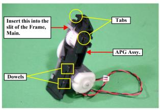
Figure 2-23. APG Assy. Installation
