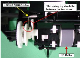
Figure 2-19. Position of Torsion Spring, 137.7
