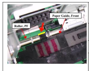
Rear of contact point between the PF Roller and tab of the Paper Guide. Front
