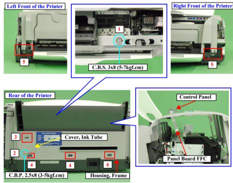
Figure 2-4. Housing, Frame Removal
