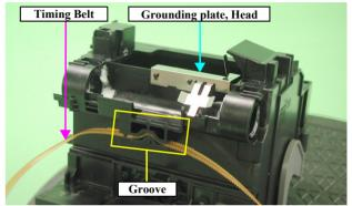
Figure 2-29. Installation Position of the Grounding Plate, Head
