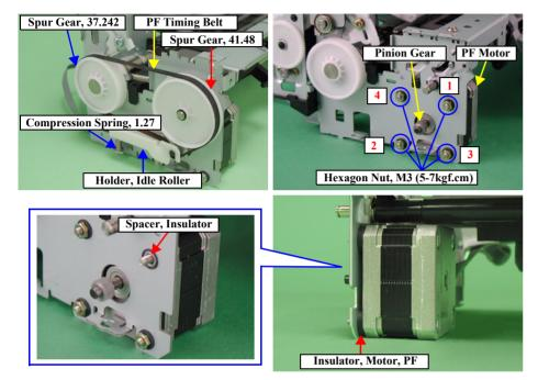
Figure 2-48. PF Motor Removal
