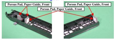
Figure 2-46. Porous Pad, Paper Guide, Front and Porous Pad, Paper Guide, Front, Support
