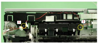
Figure 2-21. Holder, Shaft Assy. Reinstallation
