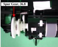
Figure 2-20. Spur Gear, 36.8 and Combination Gear, 27.2, 19.2
