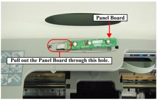
Figure 2-6. Panel Board Reinstallation
