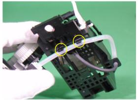
Figure 2-43. Installation Position of the Ink Tube
