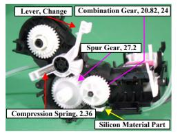
Figure 2-41. Ink System Unit Removal
