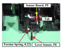
Figure 2-17. Holder, Shaft Assy. Removal (2)
