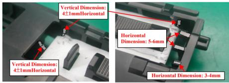
Figure 2-14. Gluing point of the Porous Pad, Paper Guide, Front
