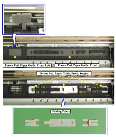
Figure 2-13. Porous Pad, Paper Guide, Front Removal
