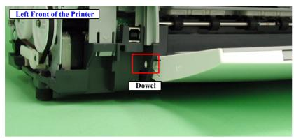
Figure 2-3. Stacker Assy. Removal
