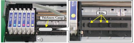
Figure 3-7. Setting the Thickness Gauge
