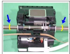
On the CR Guide Shaft outer the bearings of the Carriage
