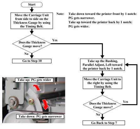
Figure 3-11. PG Checking (1)
