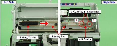
Figure 2-11. CR Motor Removal
