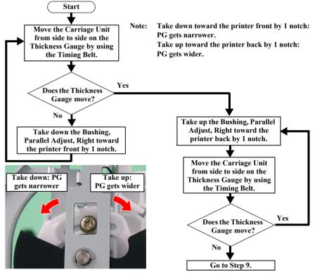
Figure 3-10. PG Adjustment (Right Side)
