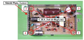
Figure 2-39. Power Supply Board Removal
