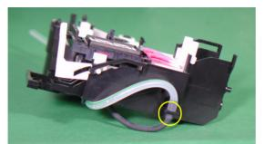
Figure 2-42. Connecting Point of the Ink Tube.
