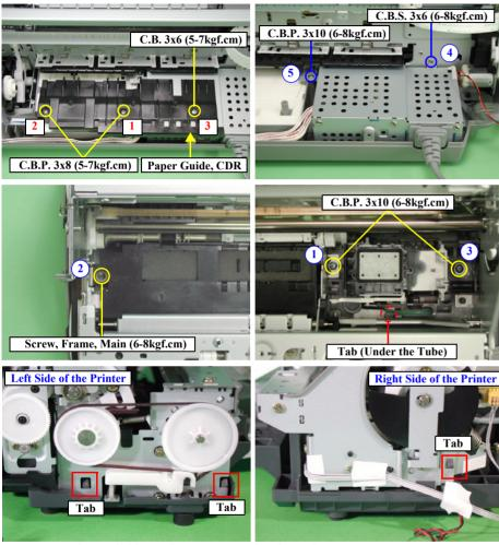
Figure 2-32. Printer Mechanism/Housing, Lower Removal
