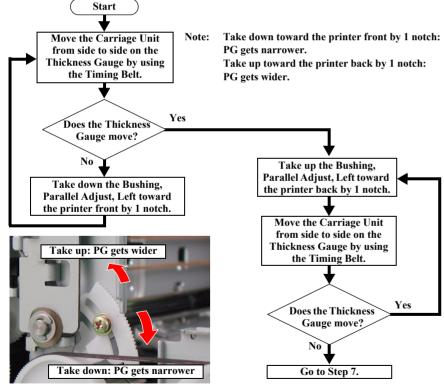
Figure 3-8. PG Adjustment (Left Side)
