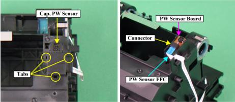
Figure 2-27. Carriage Unit Removal (2)
