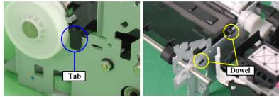
Figure 2-47. Paper Guide, Front Installation
