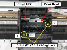
Figure 2-12. Print Head Removal
