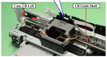
Figure 2-26. Carriage Unit Removal (2)
