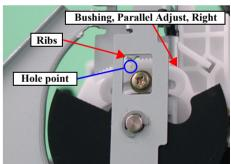
Figure 3-6. Setting the Bushing, Parallel Adjust
