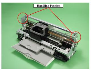
Figure 2-33. Handling Position of Printer Mechanism
