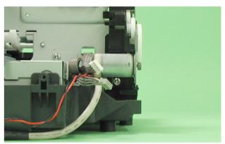
Figure 2-49. Cable connector of the PF Motor
