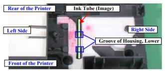
Figure 2-36. Installation Position for the Ink Tube
