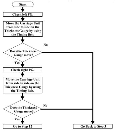
Figure 3-12. PG Checking (2)
