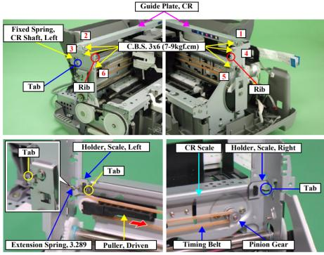
Figure 2-25. Carriage Unit Removal (1)
