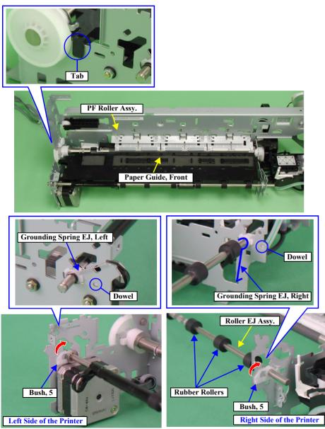
Figure 2-45. Paper Guide, Front/Roller EJ Assy. Removal (2)
