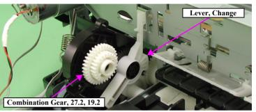
Figure 2-37. Lever, Change and Combination Gear, 27.2, 19.2
