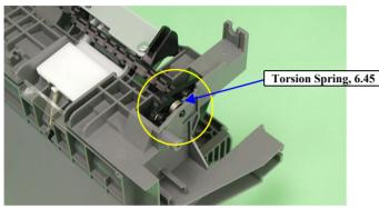
Figure 2-8. Torsion Springs, 6.45 installation
