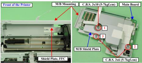
Figure 2-15. Main Board Assy. Removal
