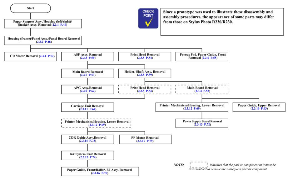
Figure 2-1. Disassembly Flowchart
